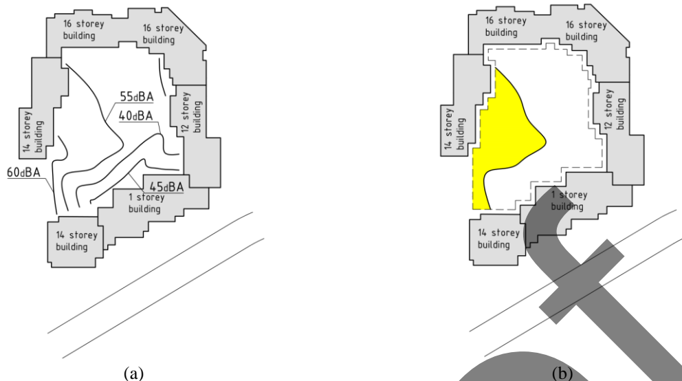
FIGURE 4. Noise level isolines in the territory of the yard (a) and the yard space of the residential building, where these regulations are not met (b)
