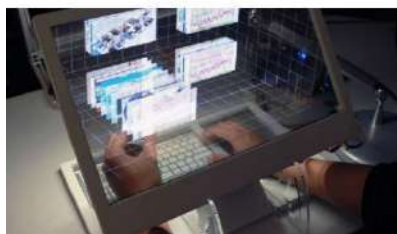
22. Microsoft's see-through 3D display using Samsung OLED screen © Silva 2014 "Glassist ..."
